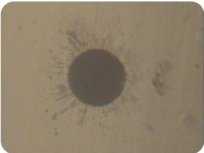
248nm, showing spatter of ejected material in this weak absorber
