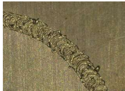
Figure 2: Brass alloy welding with beam shape and vacuum
