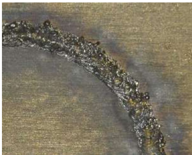
Figure 1: Brass alloy welding with beam shape without vacuum
