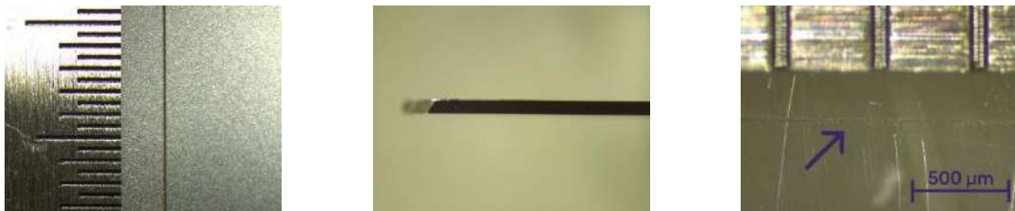
Fig. 2 Processing tests: Scribe in silicon wafer (left), cleaved wafer edge (middle), and scribe in PMMA (right).
