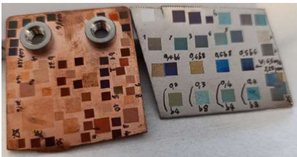
Figure 1 (a) Typical parameter grid used for laser process optimization, shown here for coloring purposes on copper and titanium. (b) Convergence plot for a 6-variable optimization of a test function, comparing different acquisition functions for Bayesian optimization.
