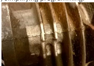
Figure 2 laser cleaning, rust on steel. Complex shape treated with no adaptation of the working distance.
