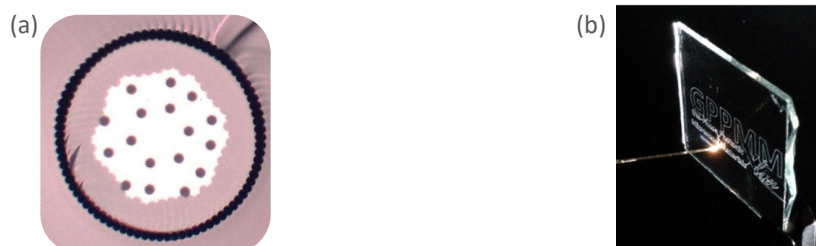
Figure 1 (a) The image shows the fibre-cross section of a fiber with an aperiodic design. (b) The image shows a USP-laser engraving on a glass slide where the beam was delivered directly from the output tip of a 10 m-long HC-PCF in a manner similar to pen writing.
